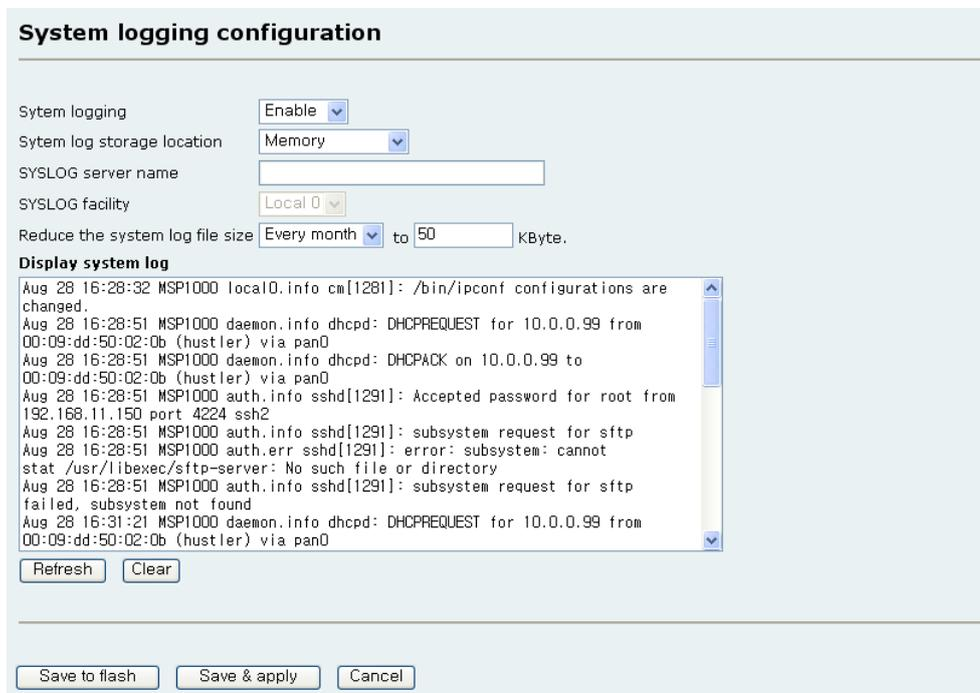
*Figure 8-2 System logging configuration*
