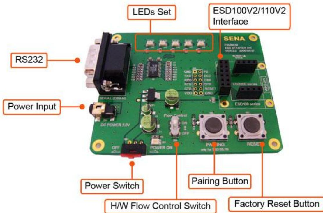
Figure 2-1 The Panel Layout of Development Board
